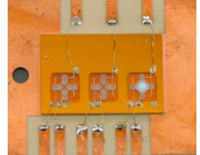
This photo shows an array of 3 thermopile sensors (3X actual size). The one on the right is coated with a material that senses ammonia vapor. Coatings for other vapors are under development.
