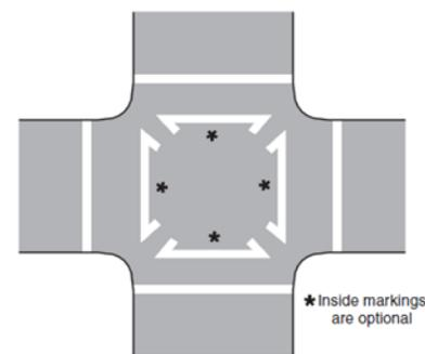
*Crosswalk markings for an all-pedestrian signal phase intersection*
