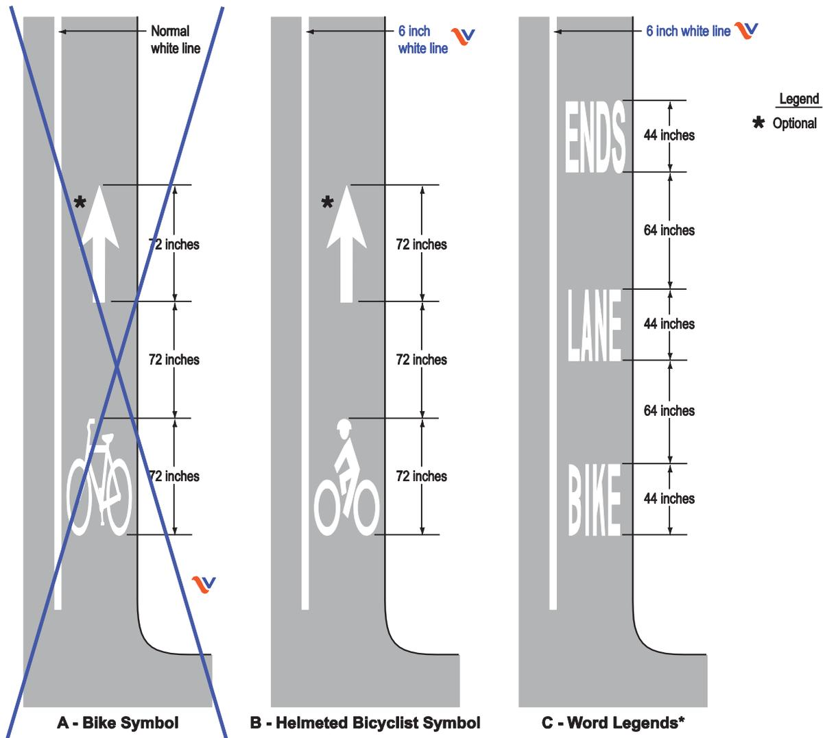
Note: Drawing C is for placement details of word legends when used. However, word legends may be utilized in addition to, but not substituting for, the Helmeted Bicyclist symbol which is required.
