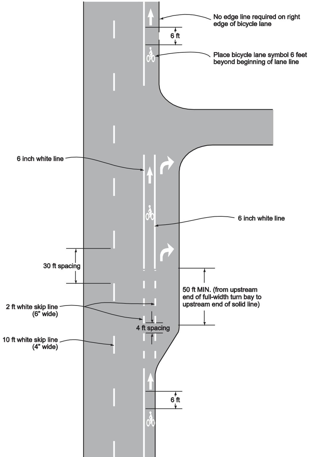
**Figure 9C-3(VA). Word, Symbol, and Arrow Pavement Markings for Bicycle Lanes**
