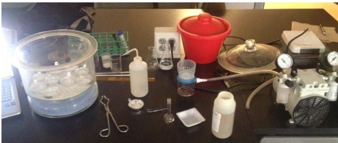
Figure 19. A picture of the total suspended solids process of filtering our samples through individual filters.
