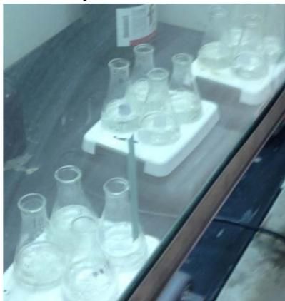
Figure 16. This depicts the digesting process where the samples and standards are on hot plates in the fume hood.
