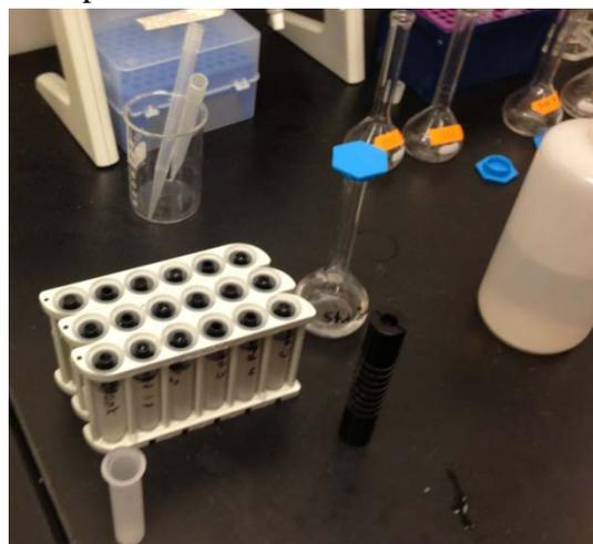
Figure 17. This displays the IC trays filled with samples and standards ready to be tested.
