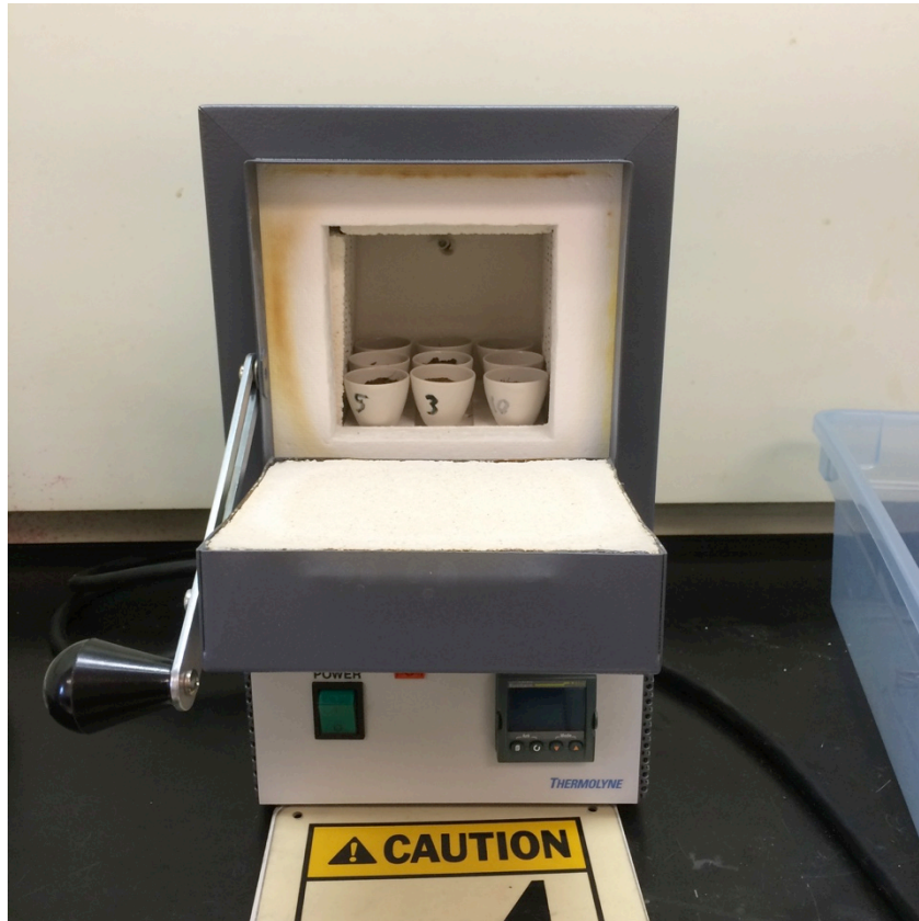
Figure 4: Muffle Furnace Used for Drying and Burning
