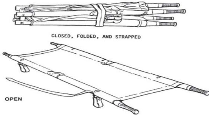
14. A multihinged folding litter (referred further in the text as a multihinged litter, or litter), is often used in tactical situations where compact size is valued. When unfolded, the litter approximates the dimensions of a standard litter.
