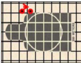
Turning the front post counter-clockwise or the opposite of the arrow will cause the bullet to impact lower, or down.
