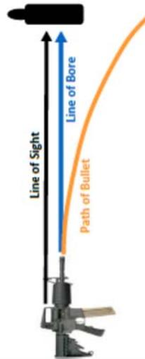
The example above is what happens when a bullet leaves the bore of a rifle in which the barrel is horizontal to the ground and the line of sight is parallel to the line of bore.
