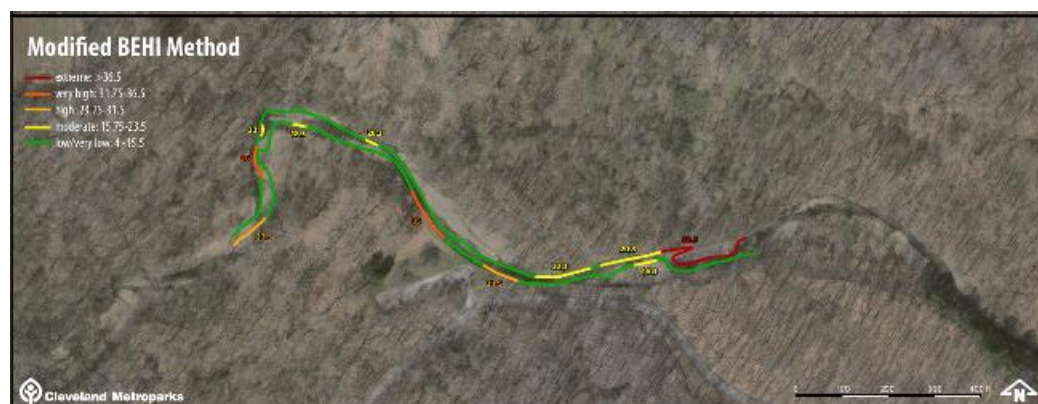
Figure 8. An example of an end product the university will have once campus streams have been assessed using a modified Bank Erodibility Hazard Index (BEHI). The modified BEHI protocol was initially developed by Cleveland MetroParks.
