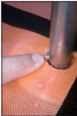
Push button to lock tower into base.
