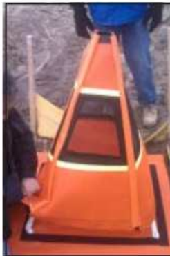
Slide tower filter over frame.
