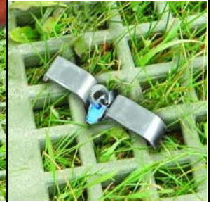
Figure 9. Loop cable back in the Gripple
