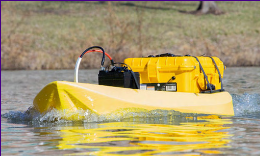
Undergrad students built an unmanned aquatic vessel to map Newman Lake's benthic levels with sonar as part of their capstone undergraduate research project (Photos courtesy of James Madison University).
