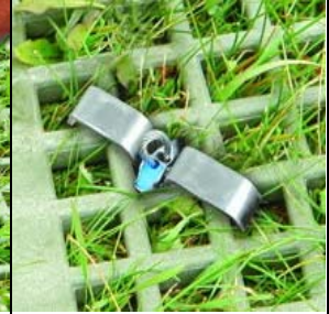
Figure 9. Loop cable back in the Gripple
