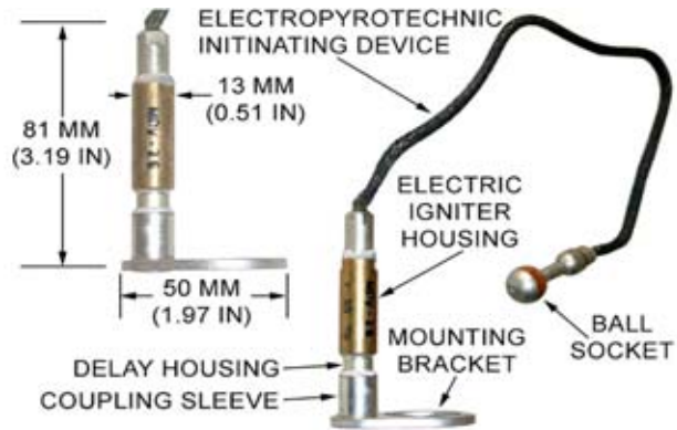
CZECHOSLOVAKIAN BOMB FUZE ARMING DELAY MECHANISM, ELECTRIC, MDV-2E
