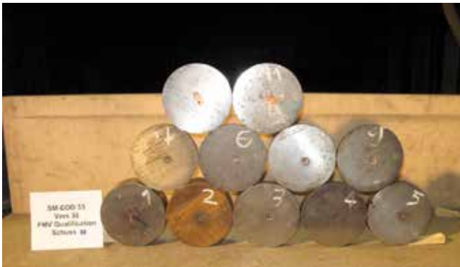
Images 4 and 5. Penetration performance witness.
