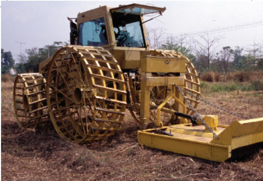
Steel wheels capable of absorbing the effects of anti-tank mines enable this machine to cut vegetation safely.
