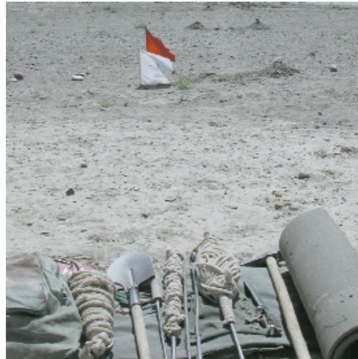
Common tools needed for mine removal.
