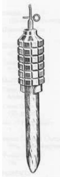
The mine body of the **PMR-1** is made from cast steel with nine rows of asymmetrical fragmentation rings. A black rubber adaptor holds the fuze.
