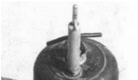
The **OZM-4** is a bounding antipersonnel mine. The mine consists of a cast-iron body, which is
