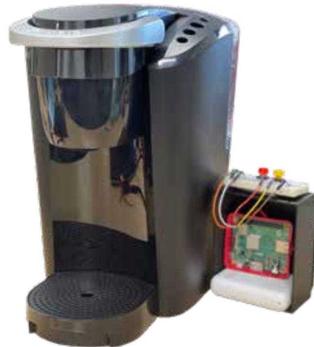
Keurig Coffee maker (left) and IoT device (right) containing Raspberry Pi connections.
