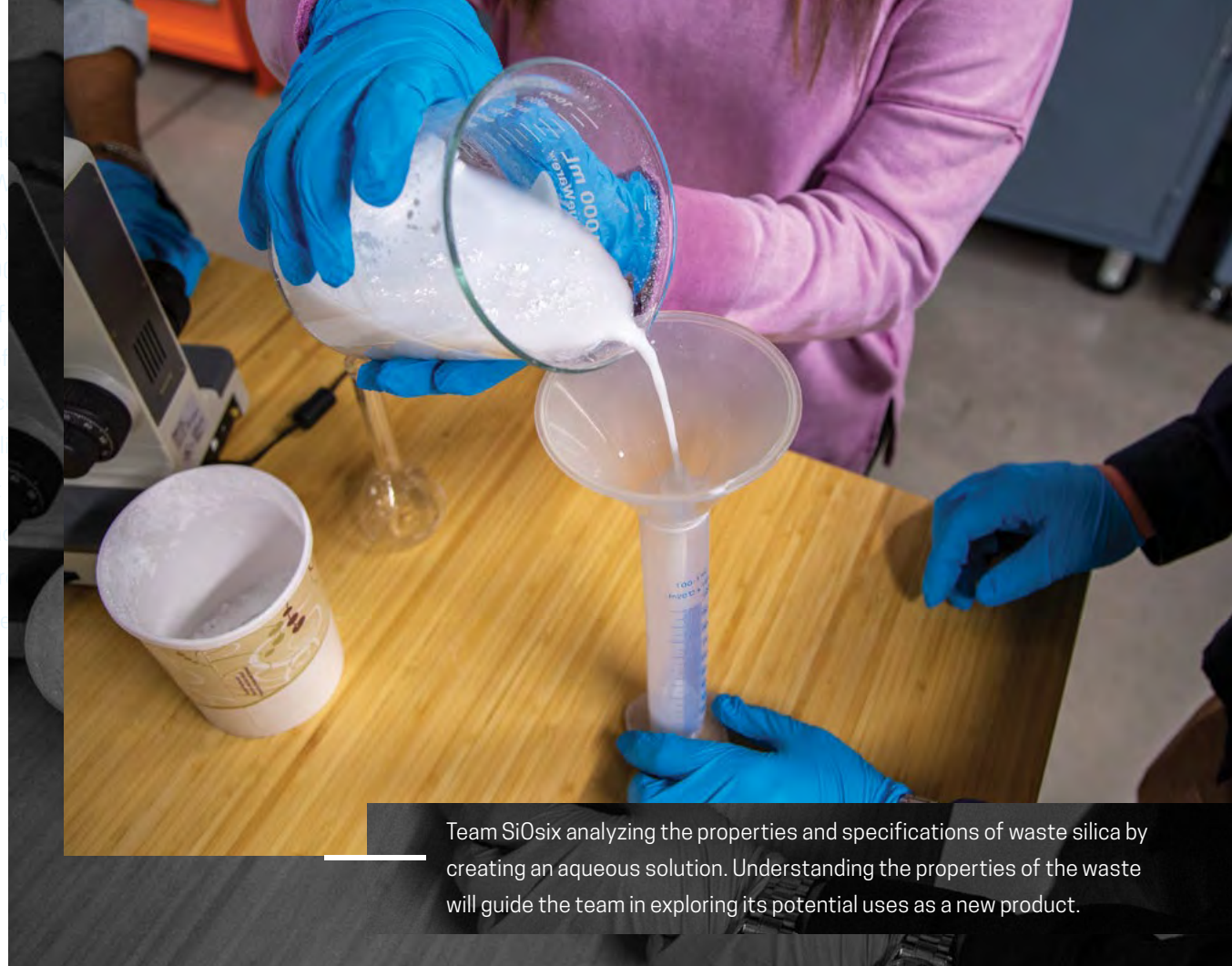
Amorphous silica (SiO 2 ) waste produced at the W. R. Grace K1 Plant in Curtis Bay, Baltimore, Maryland. Samples like this will be used to develop alternative uses for a portion of the waste produced each day from the K1 Plant.
