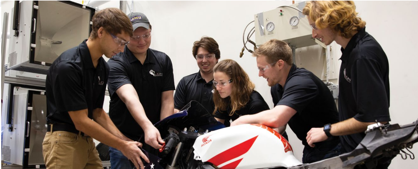
Above: The Lion team disassembles the instrumentation cluster from a donor vehicle for the purpose of installing custom gauges and rider diagnostics onto the final Lion motorcycle.
