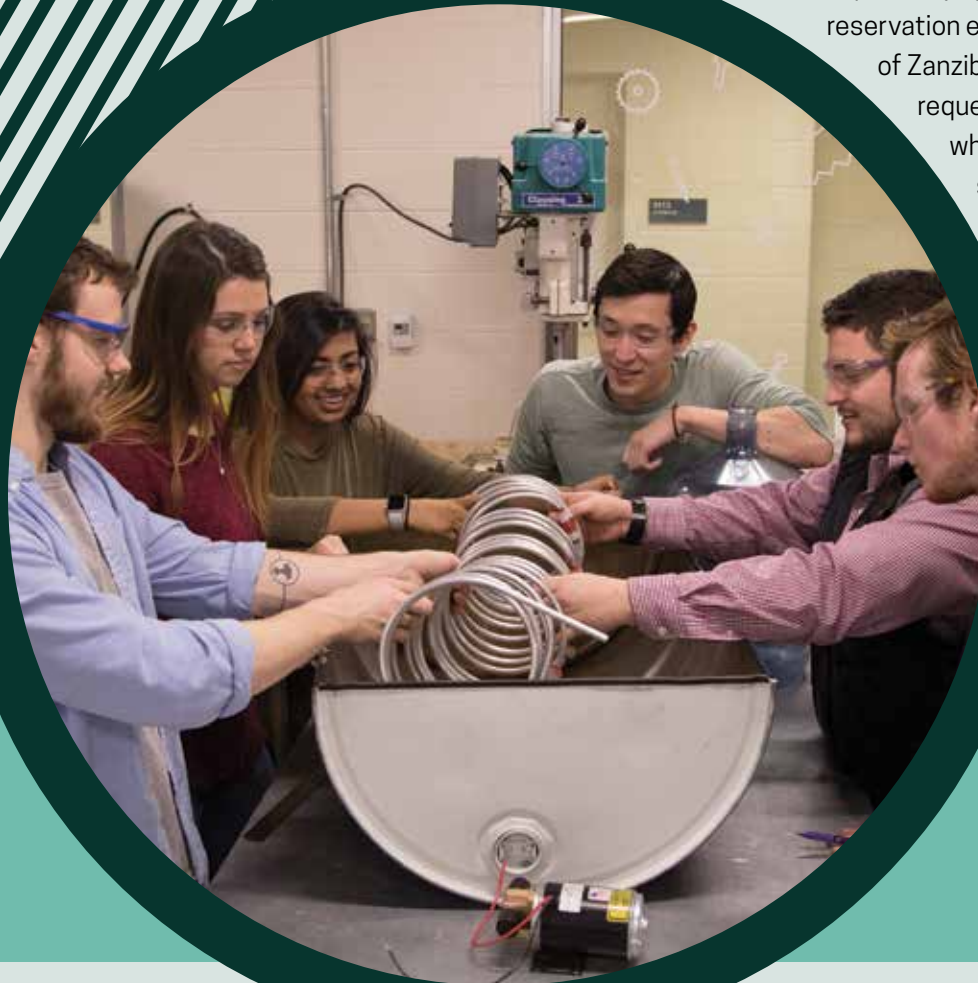
Team is mounting condenser into desalination system together.
