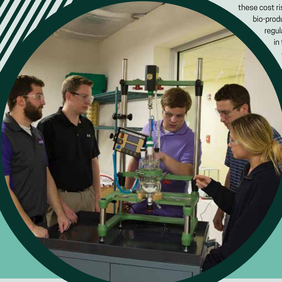
The Biopharmaceutical Production System capstone team examining the benchtop bioreactors to be used for the culturing and fermentation of several microorganisms to evaluate insulin precursor expressions.
