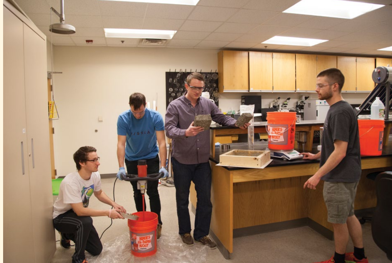
Mixing a batch of wood-aggregate concrete for highway sound walls.
