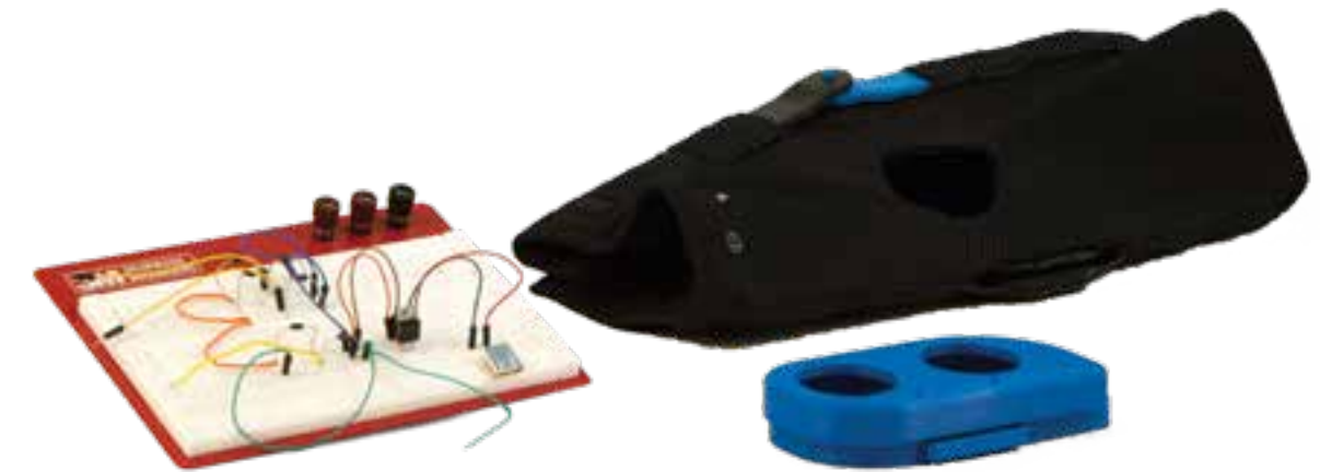
Prototype of the electrical subsystem on a breadboard (left) and knee brace (right).
