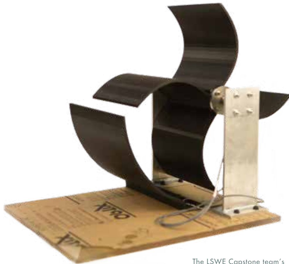
The LSWE Capstone team's first prototype model of a drag-based wind turbine, one of several design concepts.
