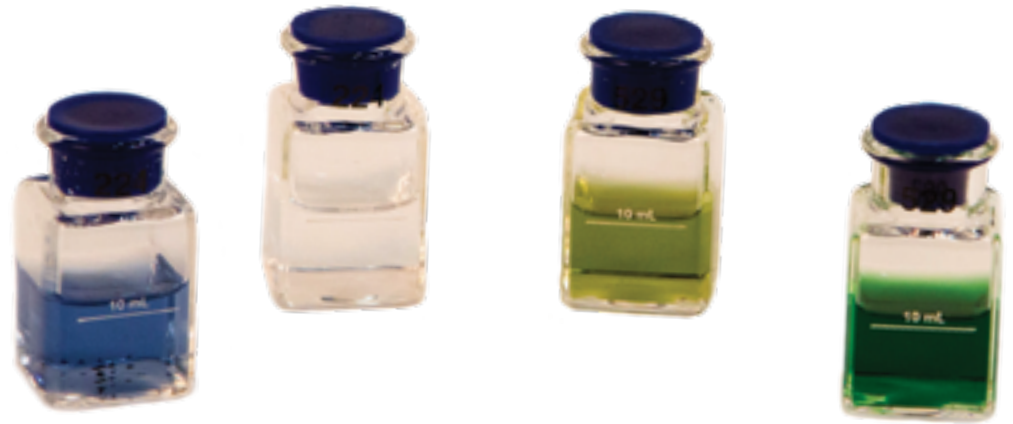
Sample vials from nutrient testing in order from left to right: Orthophosphate Sample, Orthophosphate Blank, Ammonia Blank, Ammonia Sample
