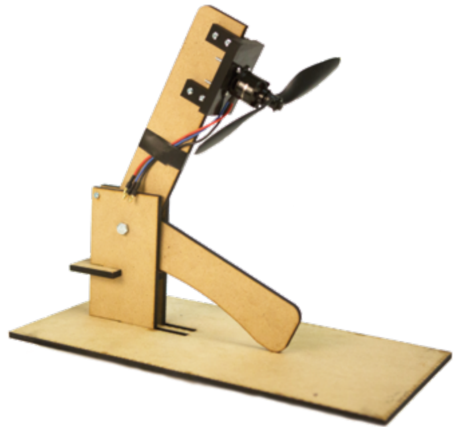
The test stand that the team will use to test the force produced by different motors and propellers.
