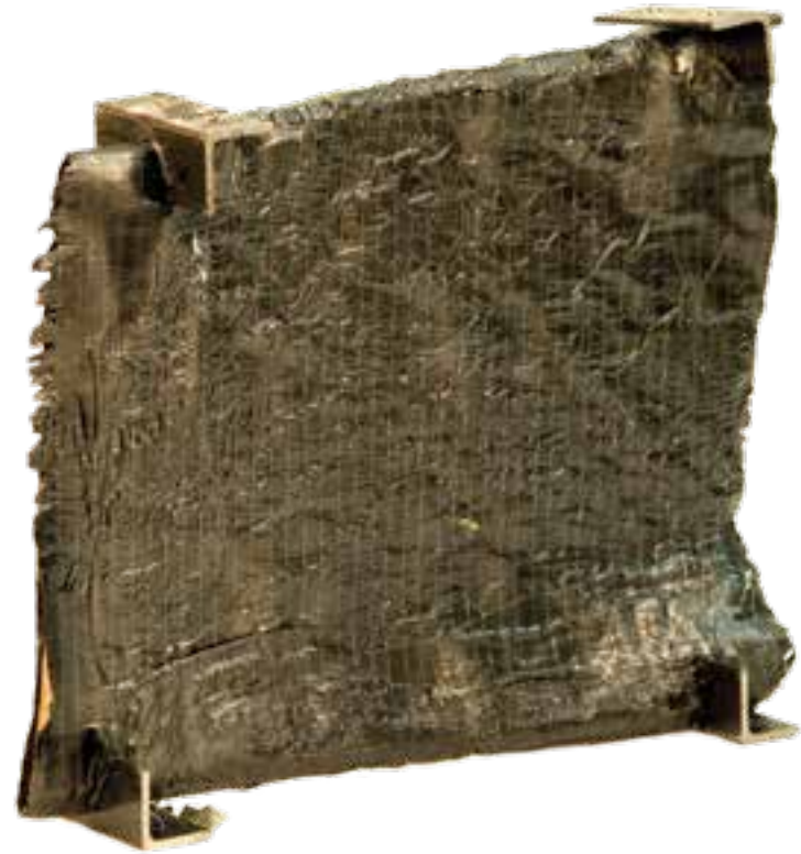
Carbon fiber-balsa wood composite leg after buckling test
