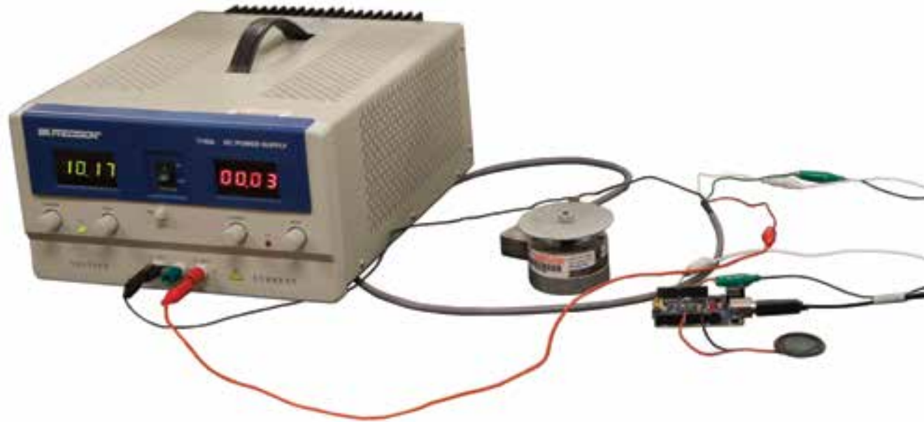
A proof-of-concept prototype was developed a child-detection device. A weight sensor is connected to a microprocessor, which alerts when a certain amount of weight is applied.
