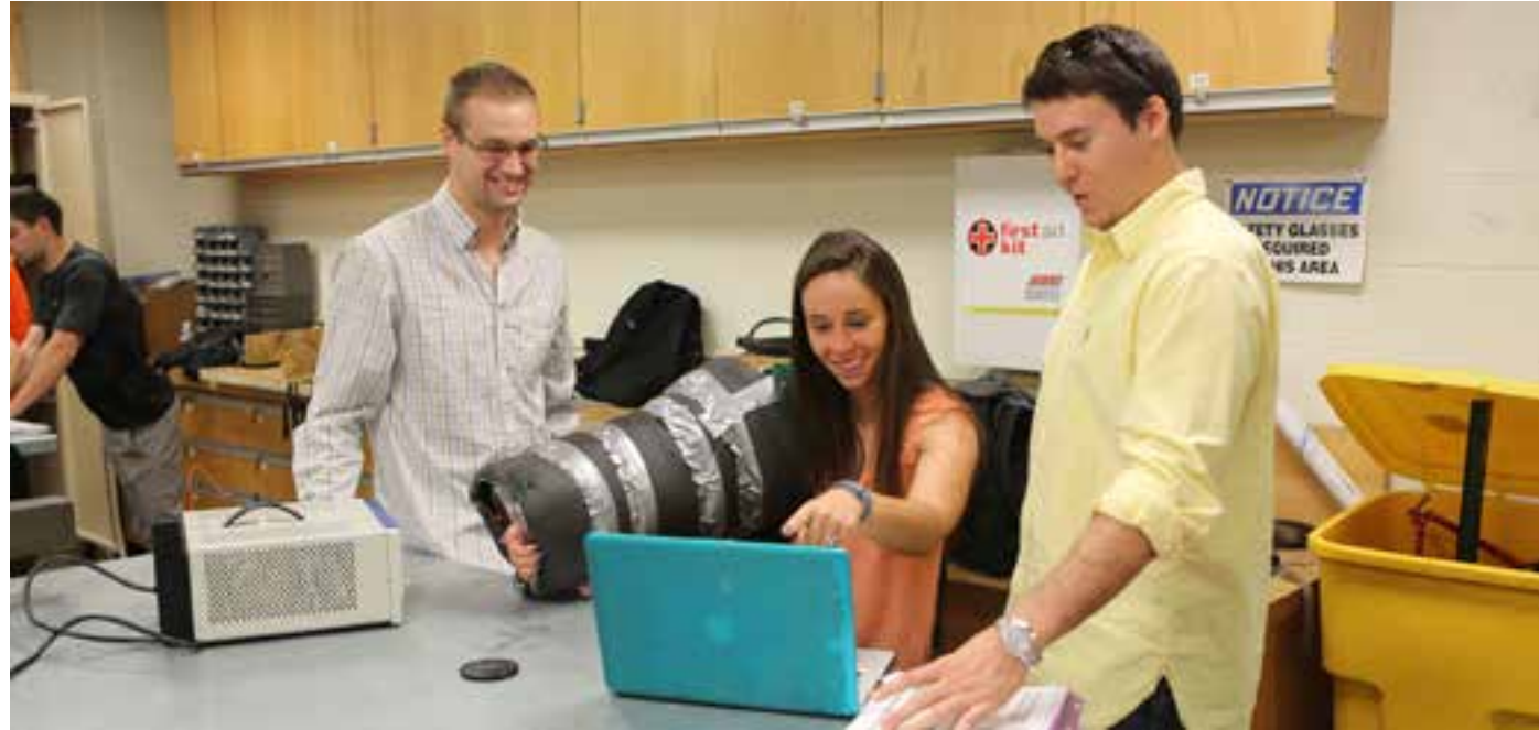
The students test the cooling apparel through simulating a hot summer day with insulated hot water flow.
