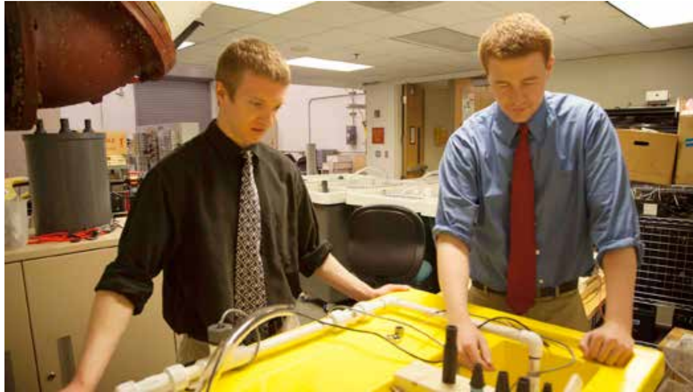
The team uses a fluid reservoir and pump to simulate full-scale conditions.
