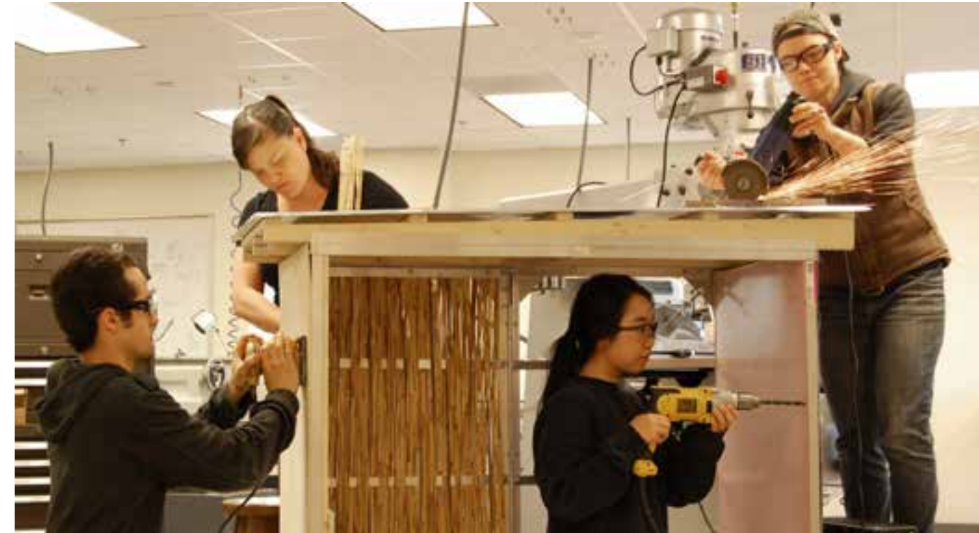
This is the team at work in the lab building a half-scale prototype of the structure. Prototyping has been the team's main method of exploring various structure designs.
