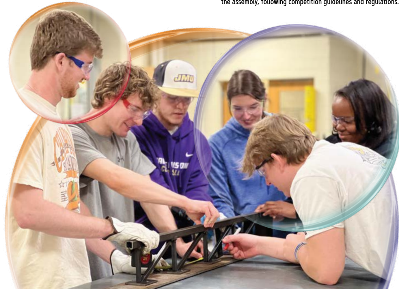
The team creating a jig to attach gusset plates to the rest of the member.
