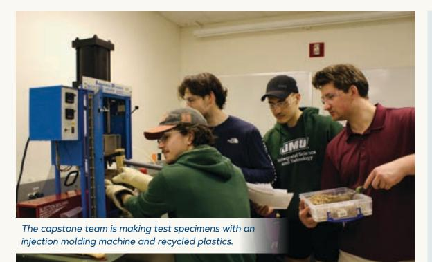
The widespread use of single-use plastics has intensified environmental pollution, making effective recycling solutions critical. This project investigates the mechanical properties of recycled polylactic acid (PLA), acrylonitrile butadiene styrene (ABS), and polyethylene terephthalate (PET) blended with bio-based fillers like rice flour, sawdust, and paper biomass. The goal is to enhance the structural integrity of recycled plastics and support the transition to a circular economy.
