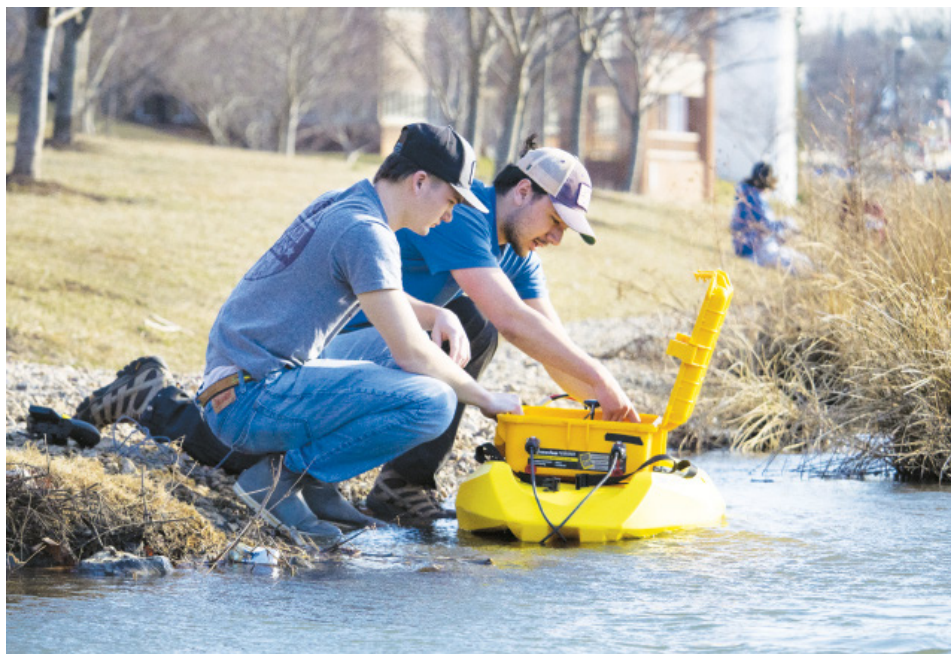
Miles McIntyre and Nathan Horner review the drone's control system to ensure it's ready to collect bathymetric data from Newman Lake.
