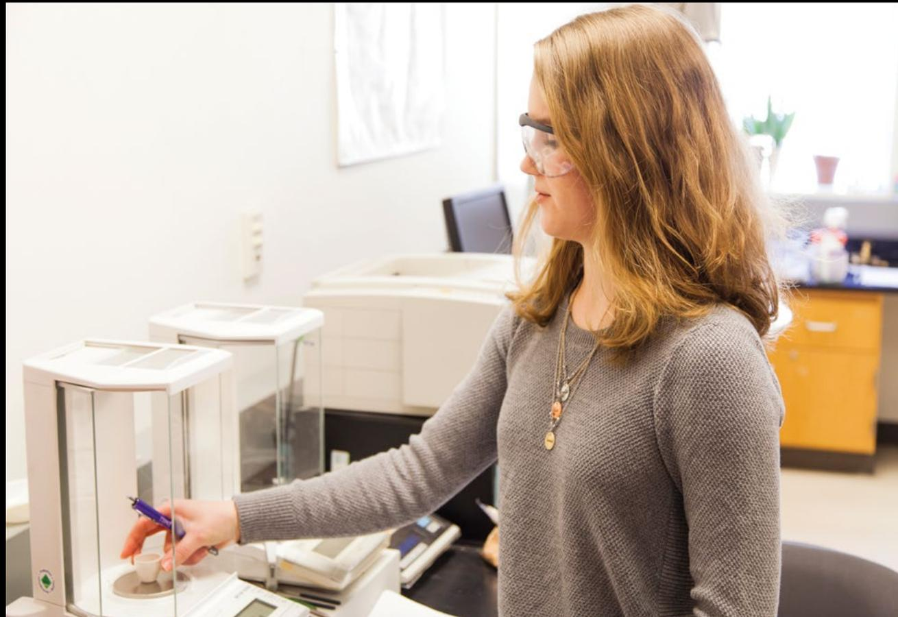
The crucibles are weighed after drying and burning to determine the percent of soil organic matter.
