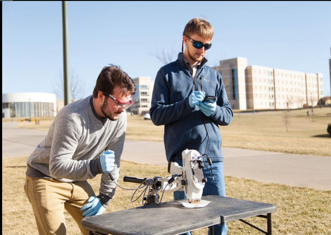
Handheld X-Ray Fluorescence Spectrometer (XRF) being used to measure the mercury concentration in soil samples from the banks of the South River in Waynesboro, VA.
