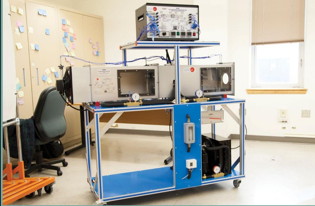
TAAB Laboratory air conditioner unit tested for heat loss and COP.
