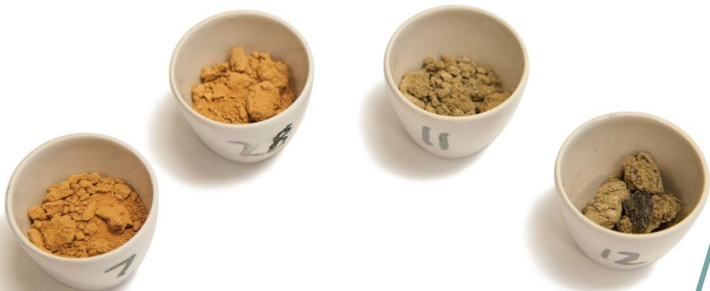
The two crucibles on the left contain soil that has been burned at 700 degrees Celsius for one hour. The two on the right contain soil that has been dried but not burned.
