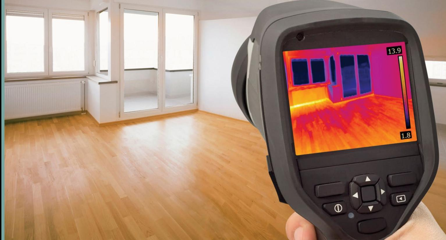
A thermal imaging camera, like the one shown, can be used to find areas of insufficient insulation during energy audits.
