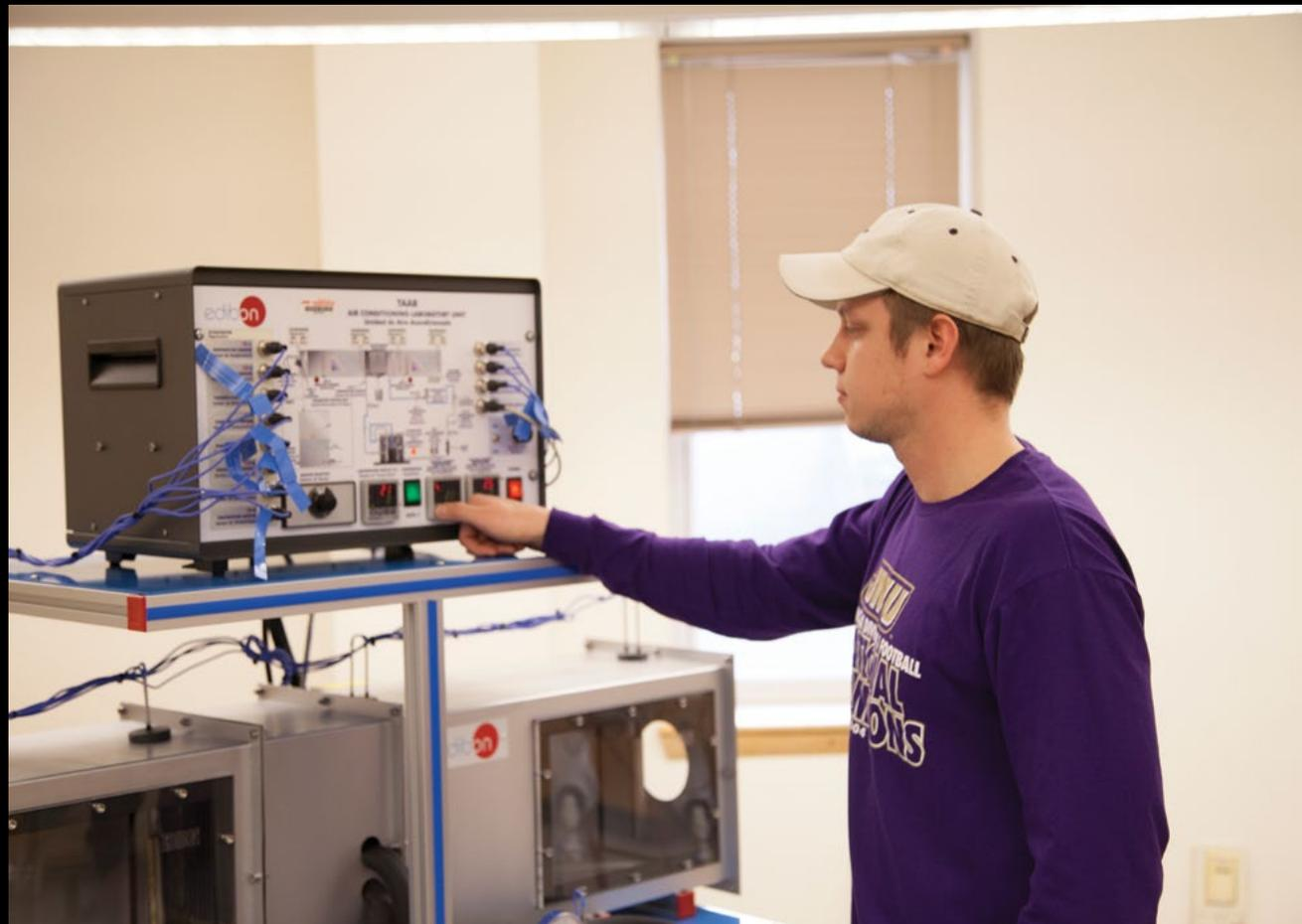
An Air-Conditioning Laboratory Unit, TAAB by Edibon® was employed in the project to investigate the system performance of an air-conditioner with different refrigerants such as R-134a, R-410A, and R-22.
