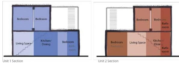
These diagrams represent the flow between the housing units, the general layout as well as the visual representation on the incremental building process of each unit.
