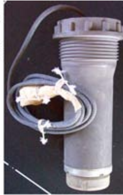
U.S.S.R. BOMB FUZE, NOSE AND TAIL, IMPACT, AVB-E
