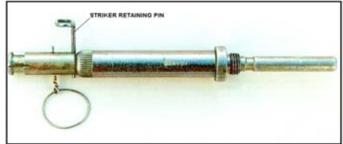
MUV-2 FITTED WITH A PERCUSSION DETONATOR ASSEMBLY
