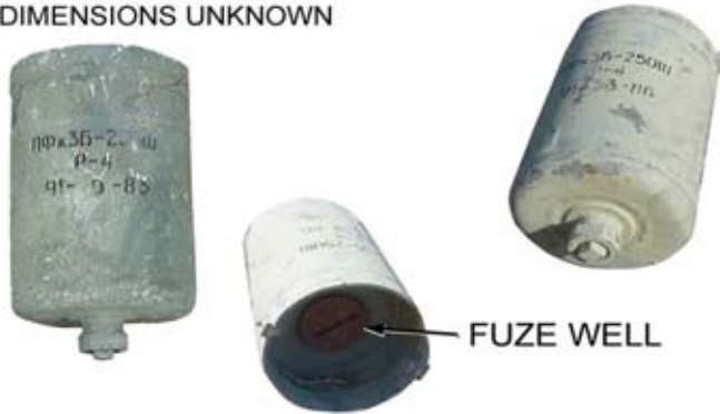
U.S.S.R. BOMB IGNITER, FIRE BOMB, PFK-ZB 250SH
