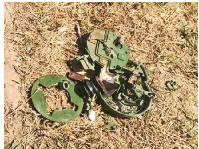
Figure 5. Result of the strike on the PMN2 with the 14mm steel slug.
