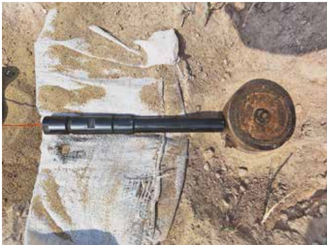
Figure 2. Mini De-Armer set up to destroy a PMN AP mine using the 16 mm, 2.4 g plastic slug. Note that a sandbag is placed on top of the tool before firing to dampen the recoil.
