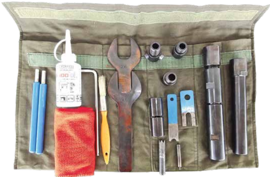
Complete Mini De-Armer with de-bulleting kit, reloading kit and tool roll. All graphics courtesy of author.
