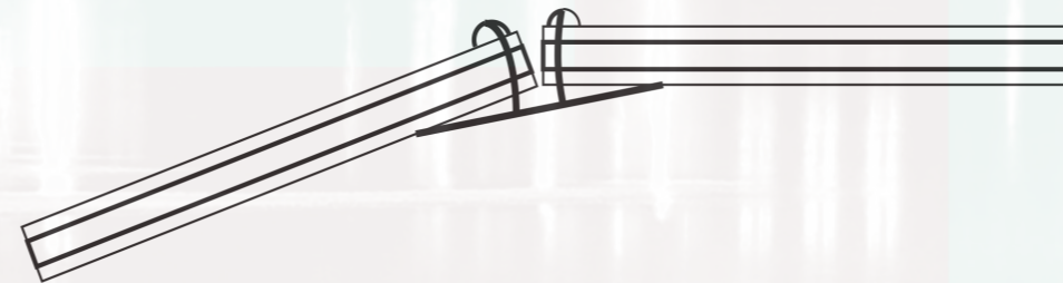
roofing cantilever in field welding panel attachment. coper-foam-copper in aluminum frame and aluminum attachment pieces.
